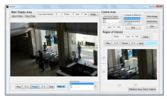
Figure 3. User interface of moving object detection system. The left-hand window is the Main Display Area, the upper-right window with parameter settings is the Control Area and the bottom-right window is the Region of Interest selected from the main scene by users through interactive tools.
