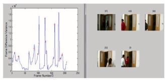
Figure 5. Frame difference variance curve and corresponding key frames with intentional illumination intensity change.
