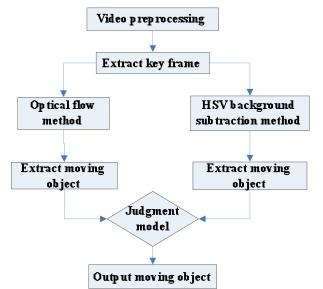
Figure 2. Hybrid moving object detection system flowchart.
