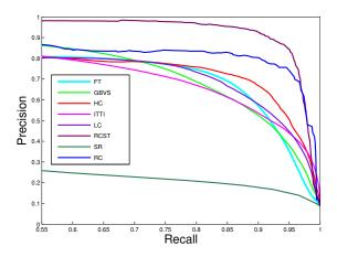
**Fig. 4**. Precision and recall curve. The RCST-based detection method yielded better detection precisions as well as higher recall values.
